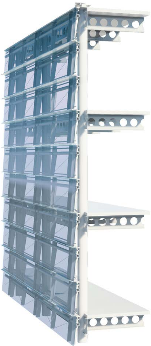
SERRATED RAIN-HARVESTING CURTAINWALL
