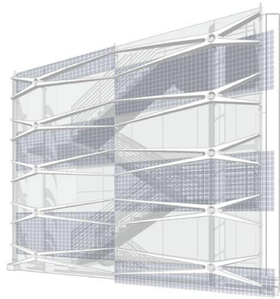
PV PANELS AT STAIR TOWERS
